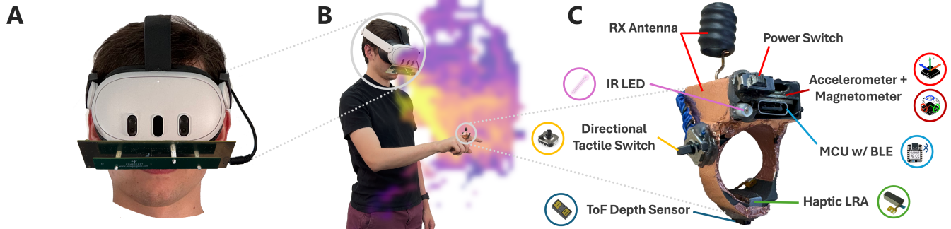
Figure 1: We developed EverRing, a smart ring that has no battery and never needs to be recharged. Instead, we use an RF transmitter incorporated into an XR headset/glasses (A), which is less battery- and space-constrained than a ring, to wirelessly power our ring (B). With less need to conserve power to extend runtime, our ring (C) offers a rich suite of input and output capabilities. For instance, as an XR accessory, it could provide eyes-free interface navigation using its directional tactile switch, use its IMU to aid in low-power hand tracking, and even provide haptic feedback when interacting with virtual widgets – capabilities not presently offered by any other smart ring, chiefly due to limited battery power.
