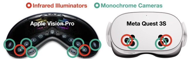
Figure 5: XR headsets on the market already include integrated infrared illuminators and infrared-sensitive cameras, suggesting EclipseTouch could be enabled via a software update. Additionally, we note that future AR glasses could also incorporate a single camera and LED in opposite corners of the frame, much like Ray-Ban Meta AI Glasses do today.
