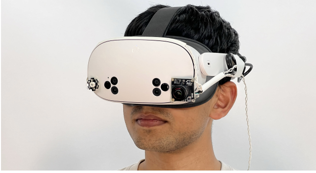
Figure 14: Based on our evaluation results, we created a final prototype featuring a single infrared emitter and camera.
