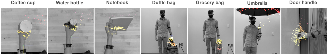
Figure 14: Example point clouds of various hand-held objects as captured by DiscoBand’s eight hand-facing depth sensors. For illustration, the real point clouds have been rotated to match a greyscale reference photo.
